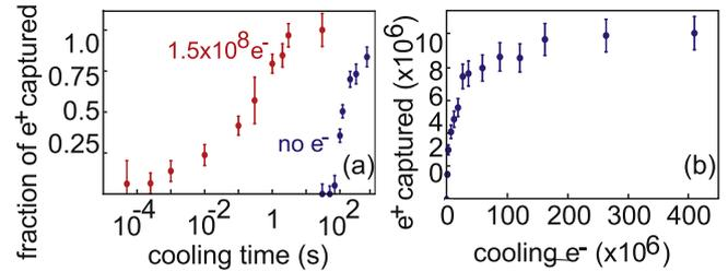
**Figure 5.** The time required for the  $e^+$  to cool is substantially reduced (a) with 150 million  $e^-$  compared to no  $e^-$  cooling. The dependence of the cooling efficiency on the number of cooling  $e^-$  is shown in (b).
