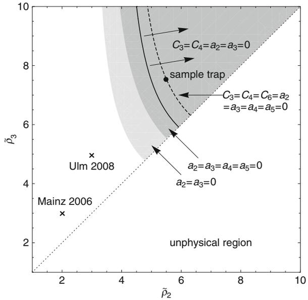
**Fig. 4 a** Amplitude dependence of  $\omega_z(A) \approx 2\pi \cdot 64$  MHz for optimized configurations of the sample trap is comparable or smaller than for the cylindrical trap. **b** Slight adjustments in the applied potentials minimize the dependence of  $\omega_z$  upon fluctuations about a large oscillation amplitude (solid) rather than for small oscillation amplitudes (dashed)
