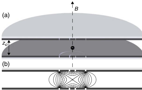
**Fig. 7** **a** A mirror-image Penning trap is formed with two planar trap electrodes facing each other. Particles can be loaded through a tiny axial hole in one of the electrodes (not visible). **b** Side view of trap electrodes and equipotentials spaced by  $V_0$ , with the infinitesimal gaps between the electrodes widened to make them visible. The equipotentials extend into the gaps between electrodes. The dashed equipotentials of an ideal quadrupole are superimposed near the trap center
