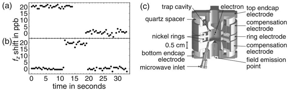
**Fig. 1** **a** QND observation of a spin flip of one trapped electron. **b** QND observation of a one-quantum cyclotron transition for one electron. **c** Cylindrical Penning trap within which the electron is suspended
