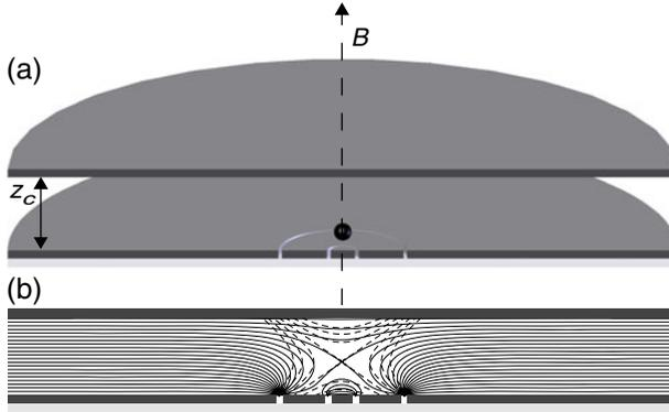
**Fig. 6** **a** A covered planar Penning trap, which could be loaded through a tiny axial hole in the cover (not visible). **b** Side view of trap electrodes and equipotentials spaced by  $V_0$ , with the infinitesimal gaps between the electrodes widened to make them visible. Some equipotentials extend into the gaps between electrodes and some terminate at infinity. The dashed equipotentials of an ideal quadrupole are superimposed near the trap center
