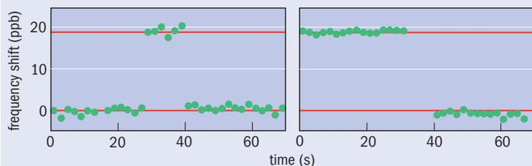
To measure the magnetism of an electron suspended in a Penning trap, the Harvard team looks for tiny changes in the electron's oscillation frequency that signal a quantum jump up to an excited cyclotron state and back down (left) or signal a spin-flip (right). Both shifts are measured in parts per billion of the oscillation frequency.
