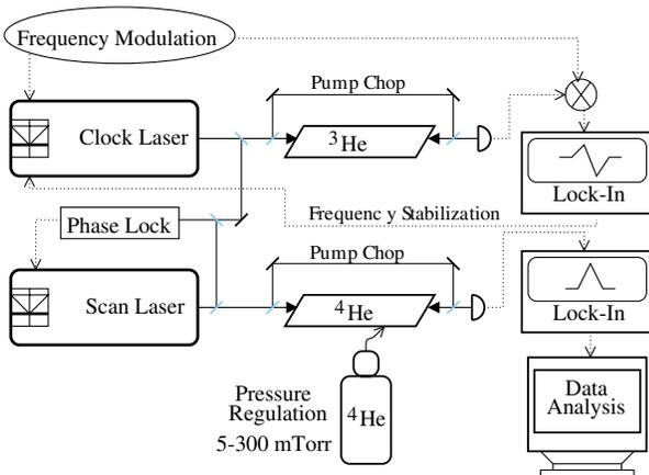
FIG. 3 (color online). Experimental setup. The 1083 nm diode “scan” laser performs saturation spectroscopy on  $^4\text{He}$ . It derives its stability from an identical “clock” laser, locked to a  $^3\text{He}$  line using frequency modulation spectroscopy.
