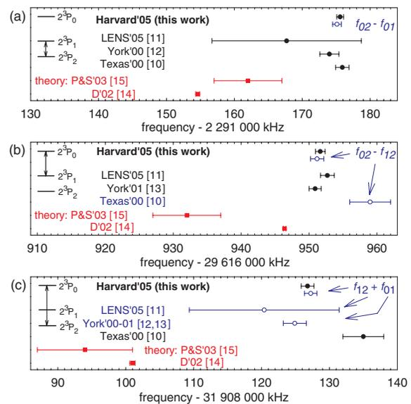
FIG. 1 (color). Most accurate measured [10–13] and calculated [14,15]  $^4\text{He}$   $2P$  fine structure intervals with standard deviations. Directly measured intervals (black filled circles) are compared to indirect values (blue open circles) deduced from measurements of the other two intervals. Uncorrelated errors are assumed for the indirect values for other groups.
