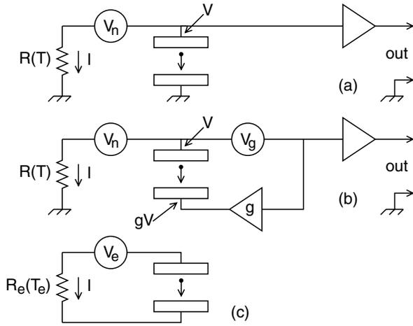
FIG. 2. Conceptual circuit without (a) and with (b) feedback. For ideal noiseless feedback,  $V_g = 0$ . For the electron, circuits (b) and (c) are equivalent.
