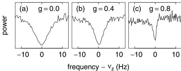
FIG. 3. Oscillator damping rate  $\Gamma_e$  (the width of the notch in the white Johnson noise) without feedback (a) and when decreased using feedback (b) and (c).
