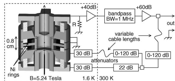
FIG. 1. Representation of trap and high frequency electronics used for feedback cooling. Static potentials applied to suspend the electron at the trap center are not shown.
