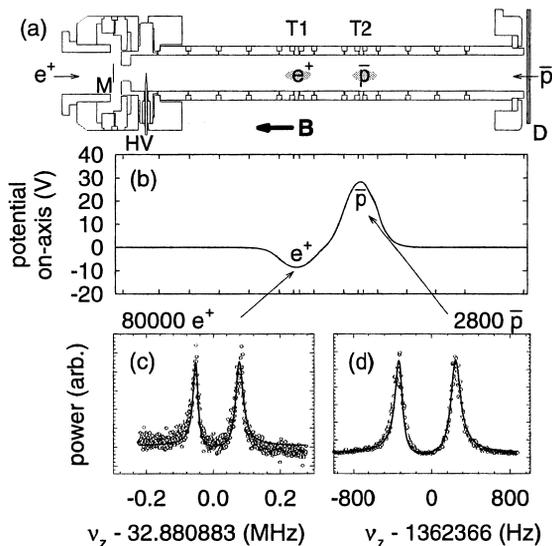
Fig. 1. (a) Electrode cross sections and the initial position of the simultaneously trapped  $\bar{p}$  and  $e^+$ . (b) Trap potential on the symmetry axis. Fits (solid curves) to the electrical signals from simultaneously trapped  $e^+$  (c) and  $\bar{p}$  (d) establish the number of trapped particles.
