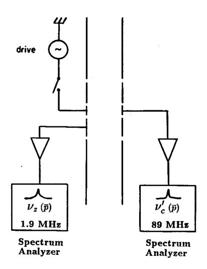
Figure 7.1: Schematic diagram for antiproton (proton) cyclotron frequency measurement.
